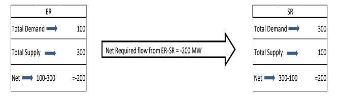
Case 2: There is congestion in ER-SR corridor and flow is constrained to 100 MW:
